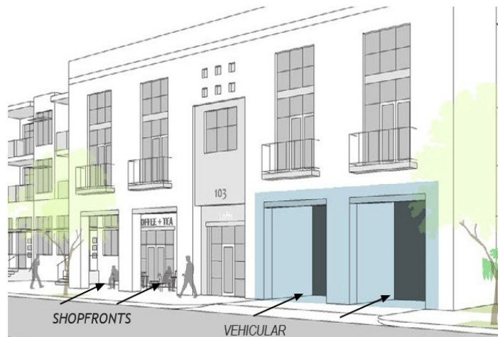
Figure 2.1-3 Parking structure and façade design
