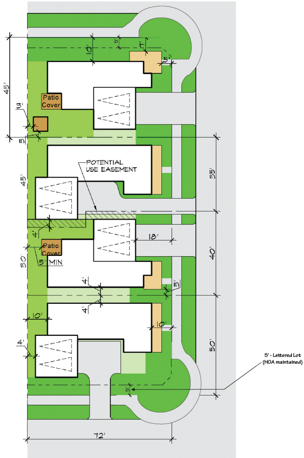
TWO-PACK OR "Z" LOT SINGLE FAMILY DETACHED *Building footprints are conceptual. Actual floor plans may differ.
